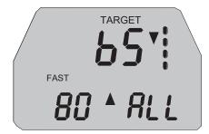
To monitor traffic in both directions (the Falcon HR will automatically indicate which direction the strongest and fastest vehicles are traveling), repeatedly depress the MODE switch until "ALL" is displayed in the PATROL window.
