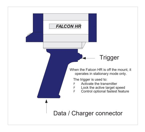
**NOTE:** The Falcon HR can connect to video systems, remote control systems, or have the operating software updated through the data connector.
