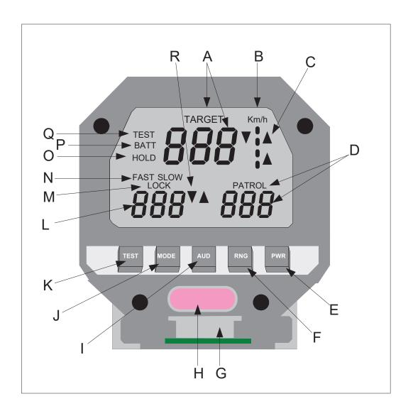
A. TARGET Displays target vehicle speeds in stationary and moving modes.
