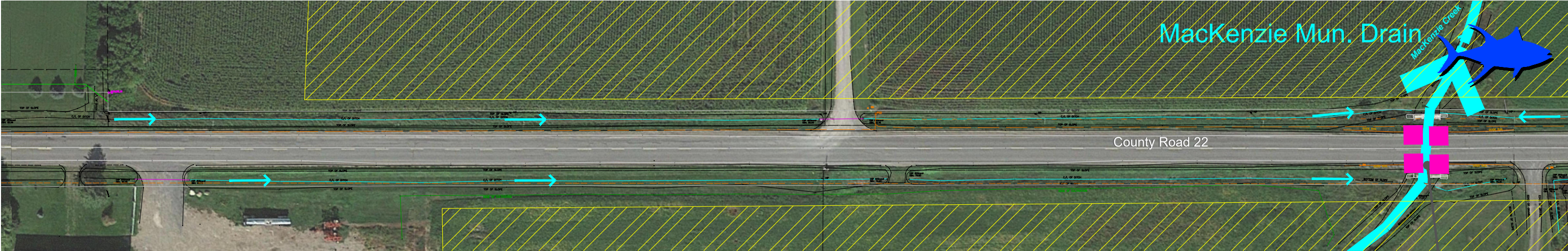
Culvert 4: Twin box culverts 38 m Steel Beam 3.3 m wide x 2.4 m ht.
