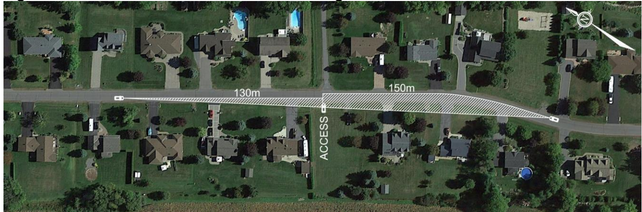
Figure 11: Steward Drive Access Intersection Sight Distance
