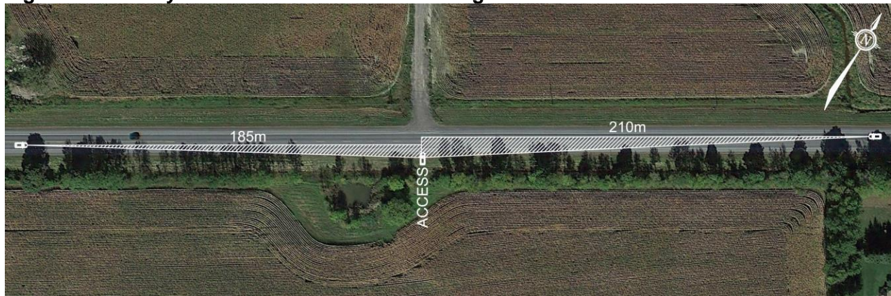
Figure 10: County Road 2 Access Intersection Sight Distance
