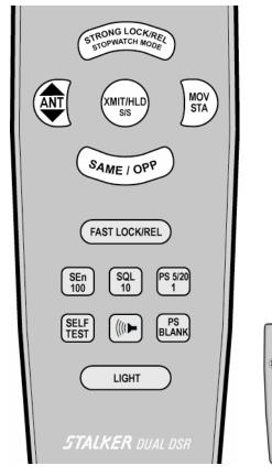
The Remote Control can be operated in wired mode by connecting a standard RJ-11 modular telephone handset cord (P.N. 155-2213-00 or Radio Shack #279-312). The cord is connected to the remote and radar unit, and battery removed for wired operation.
